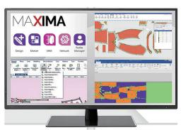
The graphic interface is customisable, as are the Shortcuts that allow a model to be created from scratch in just a few seconds. In addition, the importers of proprietary files from some of the most common cad systems make the MAXIMA system decidedly compatible and versatile. Another aspect that makes Maxima unique is the sophisticated automatic nesting algorithm that guarantees very precise efficiency rates with matchining times under a minute.
